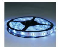
Description: • Long life.up to 30.000H • Standard pack with 5 meters/reelevery 0.5 meters as a sell unit •PCB board available for yellow PCB, white PCB •Flexible to fit different occasions every 3 lamps can be cut apart, with 3M tape on the back for easy installation Optional waterproof level: IP00/IP54 P65/IP68
